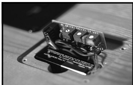
Trimpots are accessible on the rear of the guitar to set your VSC sounds.
